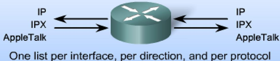
With two interfaces and three protocols running, this router could have a total of 12 separate ACLs applied.
