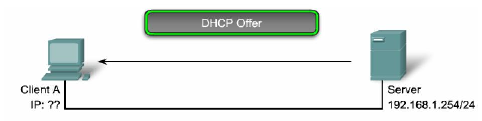
Ethernet Frame IP UDP DHCP Reply
